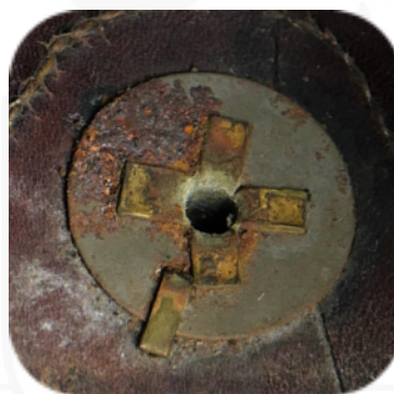
Figure 9: Example of an M/91 rosette fastening from the inside, with a pin as anti-twist device
